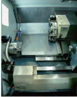
The 30° inclined bed structure employs a unique dual-layer casting process with a multi-layer reinforcing rib layout.
