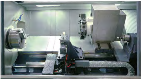
X,Z-axes box ways feature a 6-sided constraint design to achieve optimal transfer capacity and precision retention.
