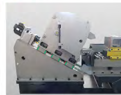
The spindle gear box feeding structure: servo motor + ball screw + linear guideway. Model 75-180 in 30° oblique cut. Model 200/230 in 15° oblique cut. Model 260/300 in parallel cut.
