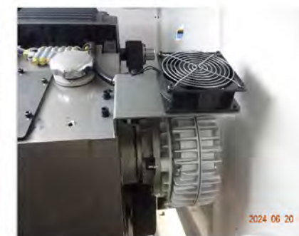
Magnetic powder brake removes all backlash for long blade life.
