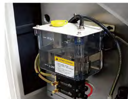
Oil mist coolant system
