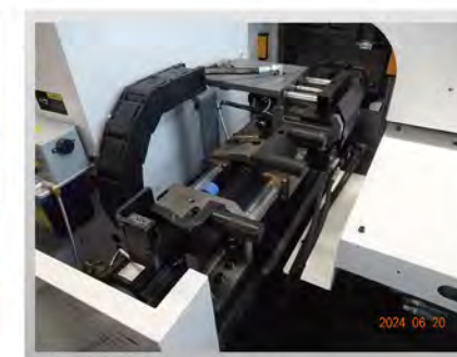
Feeding clamp(vice): servo motor + ball screw.
