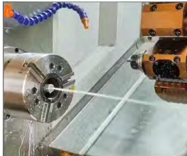
Through spindle coolant (TSC)
