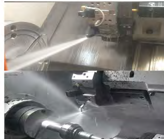
Through tool coolant (TTC)
