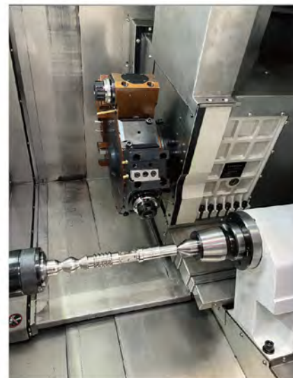
Real Y-axis (Hard Y-axis)
